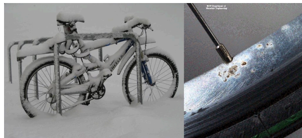
Figure 2.13 Example of galvanic corrosion on a bike in a corrosive (wet/humid/salty) environment (Hans, 2012, CC0); galvanic corrosion between chromium plated brass spoke nipple and aluminium rim (Open University, 2004, Copyright Open University)
