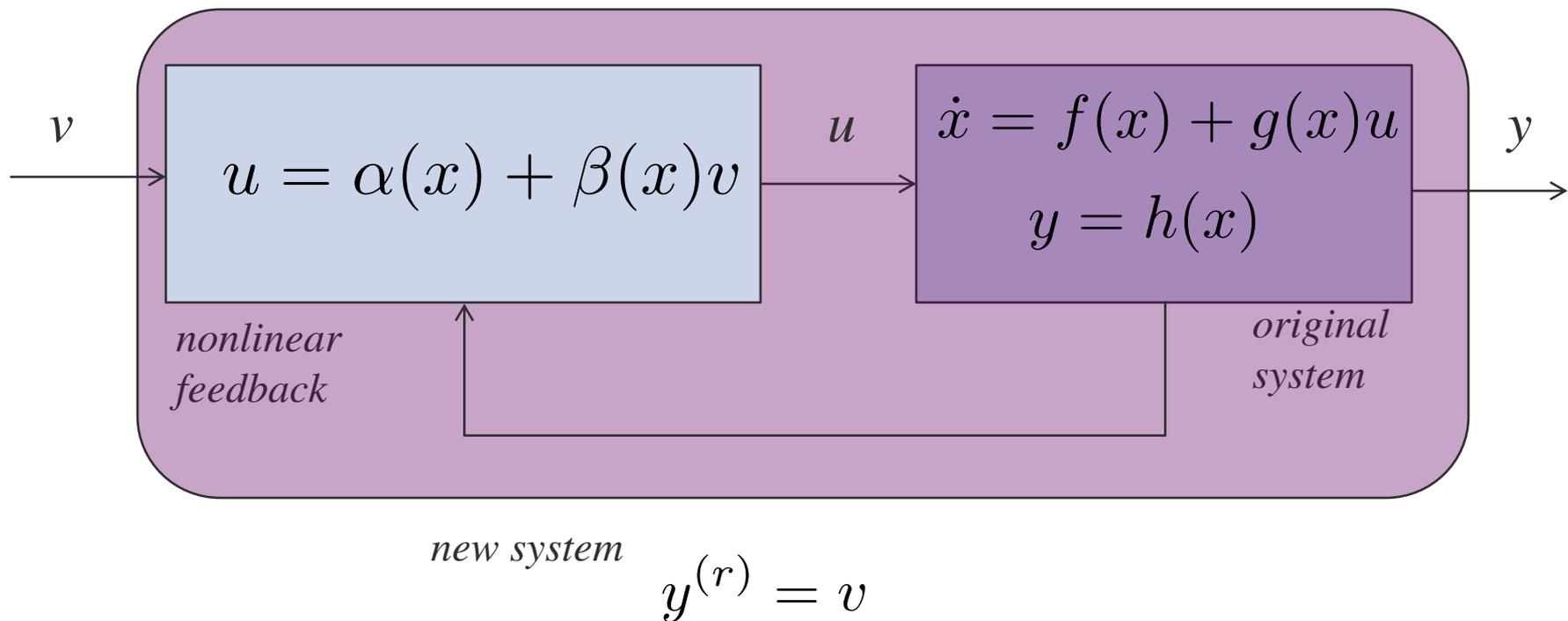
*Nonlinear feedback transforms the original nonlinear system to a new linear system*
