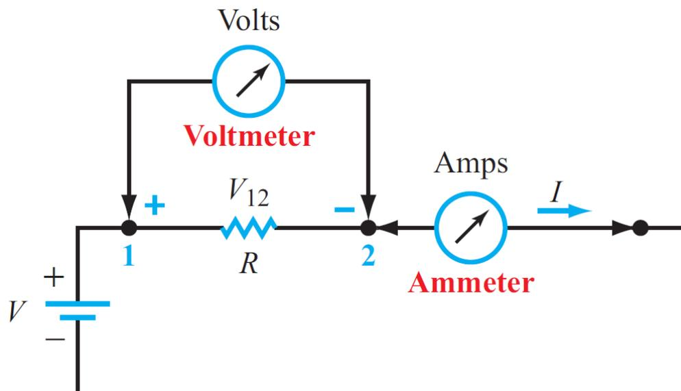
The **ammeter** is the standard instrument used to measure the current flowing between two points in a circuit. To measure  $I$  in the circuit above, we insert the ammeter into the current path.
