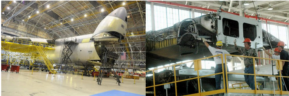
Figure 6.14 Lockheed C-5 Galaxy transport aircraft in maintenance (left) and the centre wing box of a Lockheed C-130 Hercules transport aircraft (right). Derivative of Sapp – U.S. Air Force, (2006, 2011), Public Domain.
