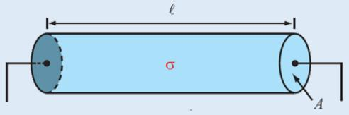
The wire in this example has a material property called **conductivity**,  $\sigma$ , which is a measure of how much obstruction the material's atoms present to moving electrons. The units of  $\sigma$  is Siemens / m. A Siemen (S) is just the reciprocal of the ohm  $(\Omega)$ . Amusingly, before being standardized, the Siemen was often called the *mho*.
