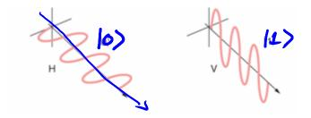
Horizontally and vertically orientated electric field oscillations.
