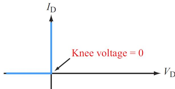
In an ideal diode, current can flow through the diode from the (+) terminal to the (-) terminal unimpeded, regardless of its magnitude, but it cannot flow in the opposite direction.
