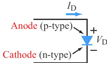
There are many types of diodes, including the basic pn-junction diode, the Zener and Schottky diodes, and the ubiquitous light emitting diode (LED) used in consumer electronics. For the present, we will limit our discussion to the pn-junction diode, commonly referred to simply as the diode.
