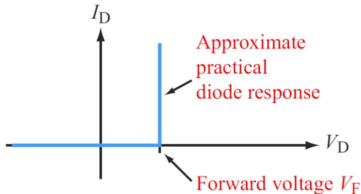
The only difference between the ideal diode model and the approximate diode model above is that in the latter the transition from reverse to forward bias occurs at a non-zero, positive value of  $V_D$ , namely the forward-bias voltage  $V_F$ . For a silicon pn-junction diode, a typical value of  $V_F$  is 0.7 V. We always should remember that  $V_F$  is a property of the diode itself, not of the circuit it is a part of.
