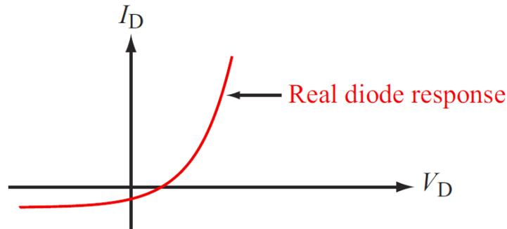
Note how nonlinear a real diode really is! For many electrical engineering applications, however, the nonlinearities are not so important, and the approximate ideal-like diode model shown below is quite sufficient.
