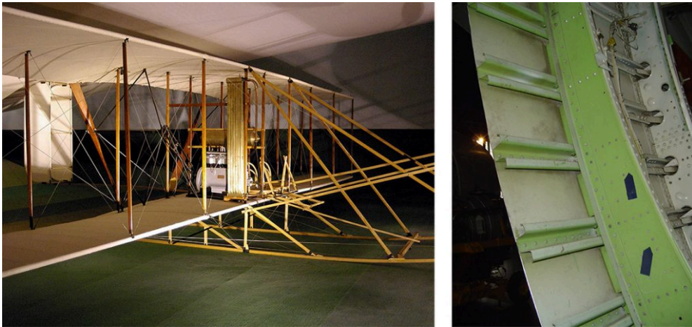
Figure 8.6 Illustration of the different design related to material usage; wood, linnen and steel trusses (left) and load bearing stiffened aluminium shell structure. Derivative from left: Cliff, (2003), CC-BY2.0 and right: Kolossos, (2006), CC-BY-SA3.0.
