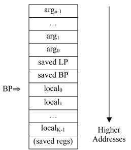
Note that BP always points to the first stack slot above the saved BP, which is the same as the first local variable (if any). It also points to the third stack slot above the first argument (if any). So within the procedure's body, its arguments and locals may be accessed via constant offsets from BP.
